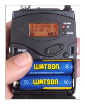
Turn both your transmitter and receiver on by pressing and holding the ON/OFF button for 2 seconds.
